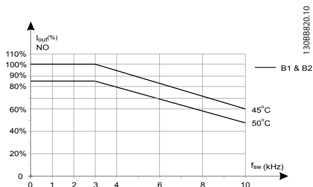
Illustration 5.10 Output Current Derating with Switching Frequency and Ambient Temperature for 600 V Frequency Converters, Enclosure Sizes B, 60 AVM, NO
