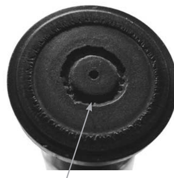
Cavitation of the piston shoes. All pistons must be replaced immediately.
