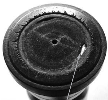
Cavitation of the piston shoes. All pistons must be replaced within the next 100-200 hours.
