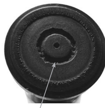
Cavitation of the piston shoes. All pistons must be replaced immediately.
