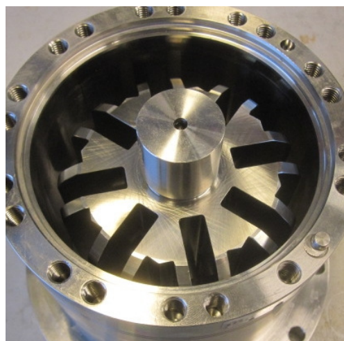
52. Gently place the rotor in the bearing
