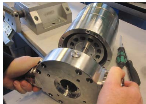
28. Position the port flange over the guide pin
