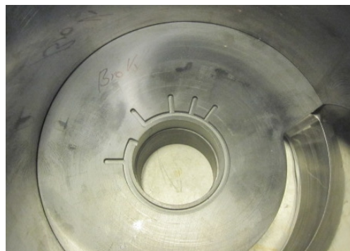
50. Position the side plate over the guide pin. NB: Make sure that the guide pin is located in the locating hole in the port plate. See #49
