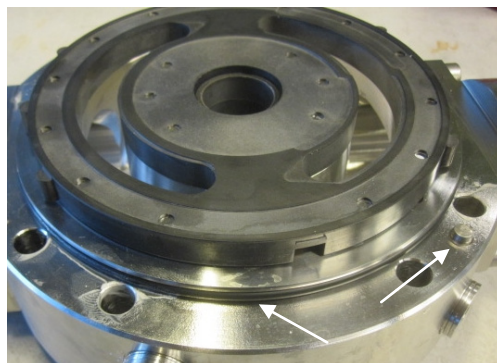
27. Change the o-ring in the flange and position the guide pin
