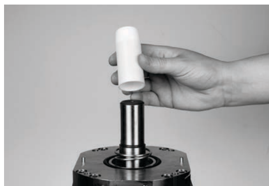
40. Mount special tool on shaft
