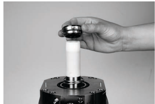
42. Mount sealing (smallest diameter pointing down)
