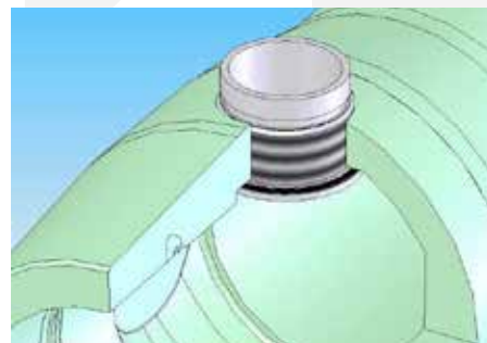
Seal seated against a flat surface
