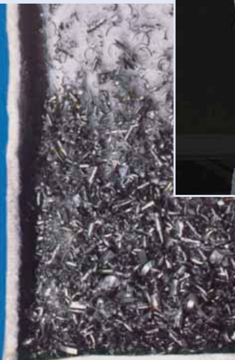
Metal fines collected from parts washer
