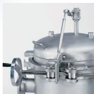
7. Close the safety interlock—housing is ready to go on-line
