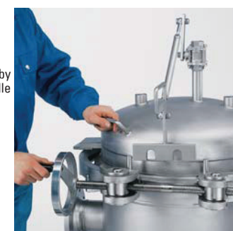
7. Close the safety interlock—housing is ready to go on-line
