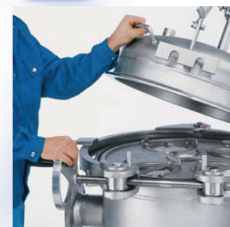
6. Close the V-clamp by rotation of the spindle
