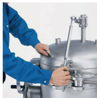
2. Rotate the spindle using the hand-wheel to open the V-clamp into the end position
