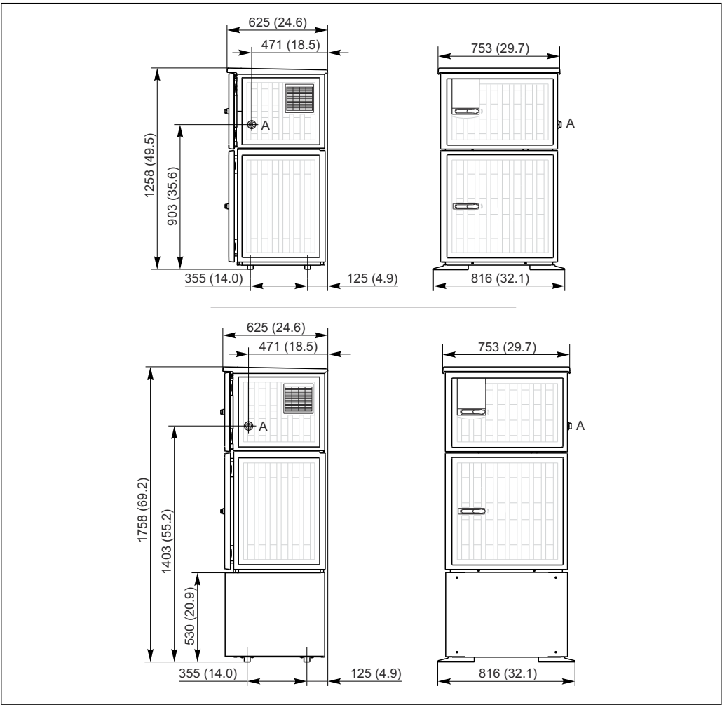
25 Dimensions of Liquistation, plastic version, without/with stand. Unit of measurement mm (in) A Suction line connection
