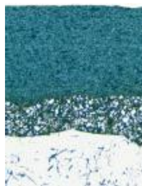
Cross section of Flygt epoxy coating
