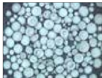
Fig. 80 Example of ARC coating type with a high reinforcing particle density
