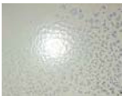
Fig. 94 Example of coated surface contaminated with PWIS
