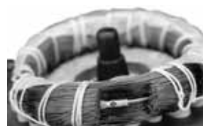
Fig. 21 PTC sensor incorporated in winding
