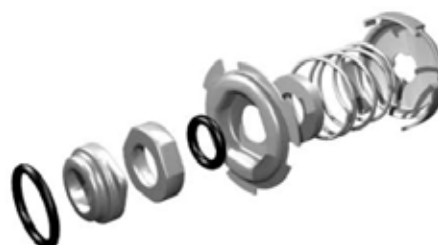
Fig. 14 Exploded view of shaft seal
