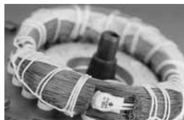
Fig. 46 Thermal switch incorporated in windings
