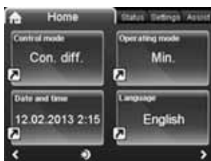
Fig. 18 Example of main display on a TPE Series 2000 with advanced control panel
