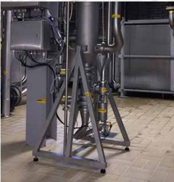
Auto-line® LE for filtration of whey in a cheese factory
