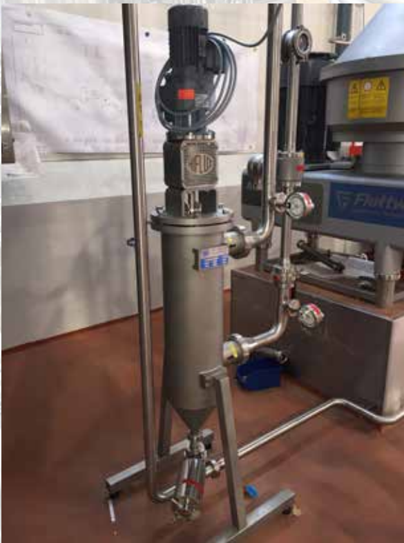
Auto-line® LR-E for filtration of gelatine water
