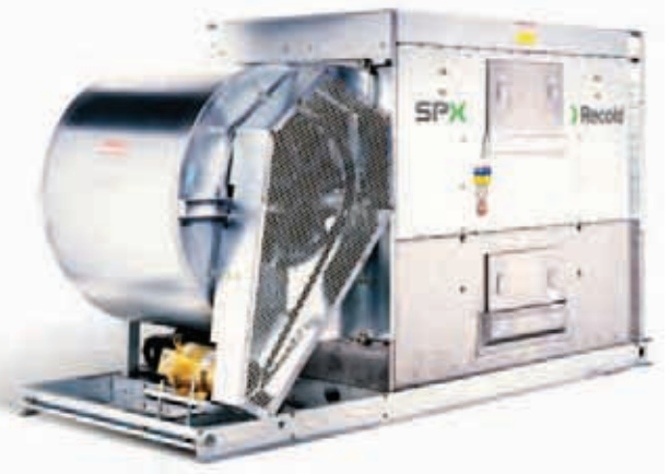
Recold JT Cooling Tower —Forced-draft, low profile design. G-235 galvanized steel factory assembled structure. Also available in 300 series stainless steel. Capacities from 30 to 415 tons per cell.
