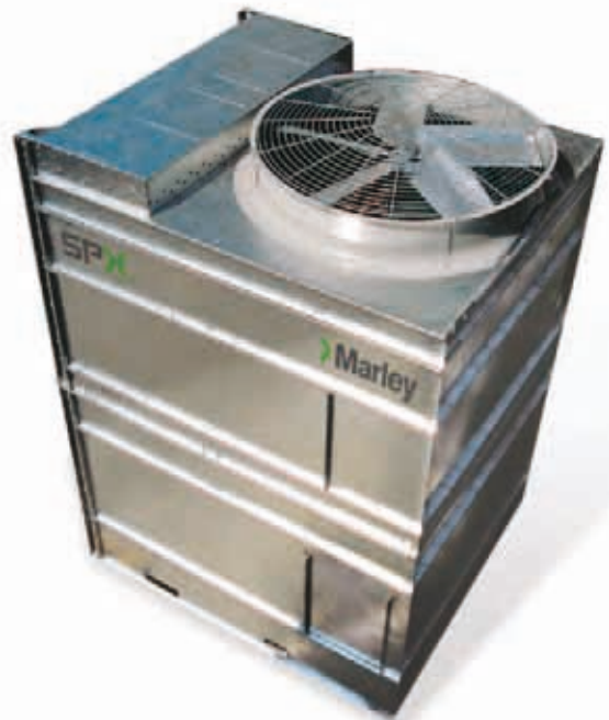
Marley AV Cooling Tower —Singleflow, induced-draft crossflow design offers pump and fan energy savings in a small footprint installation. Factory assembly and G-235 galvanized steel construction are standard. Tower cells available from 117 to 390 tons per cell. The all stainless steel option enhances the versatility of the AV. CTI Certified.
