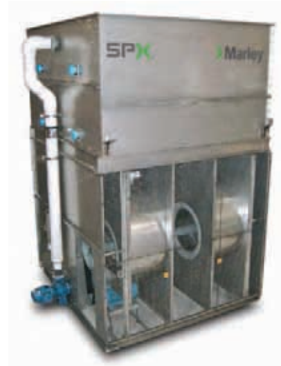
Marley MC Fluid Cooler —Forced draft, counterflow design. G-235 galvanized steel factory assembled structure. Also available in 300 series stainless steel. The ideal solution for sound- and space-sensitive applications.
