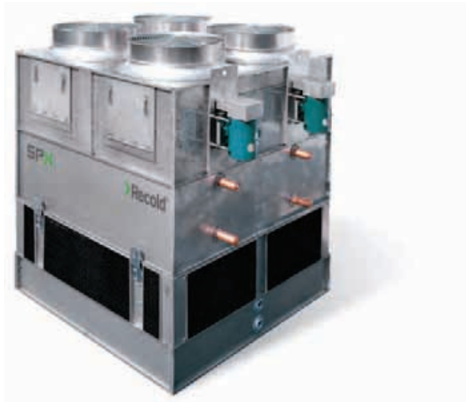
Recold MC Evaporative Condenser —Induced draft, counterflow design. G-235 galvanized steel factory assembled structure. Also available in 300 series stainless steel. Proven copper coil technology.
