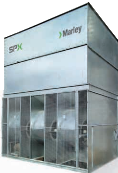
Marley Aquatower® Cooling Tower —Reliable performance has made this design the industry standard for more than 60 years. G-235 galvanized steel factory assembled structure. Also available in 300 series stainless steel construction and fiberglass construction. Capacities from 8 to 126 tons per cell. CTI Certified.
