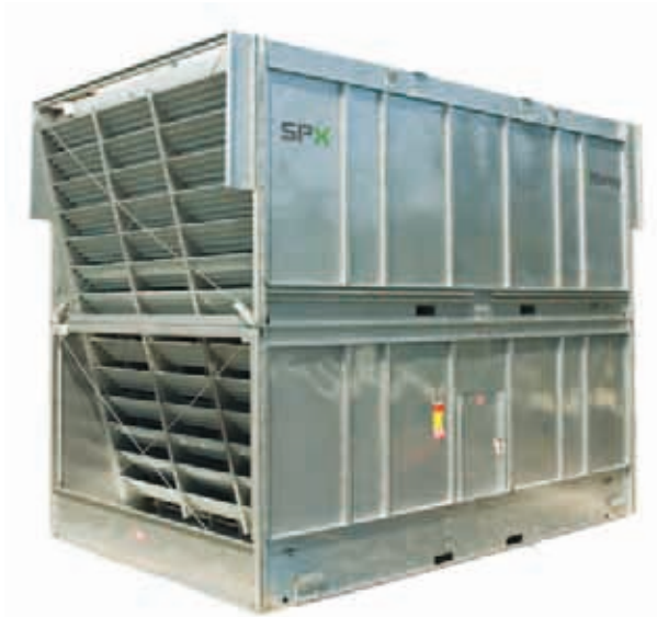
Marley NC® Alpha Cooling Tower —Splash-fill design for use at high temperature or where poor water quality prevents the use of film fill. Factory assembly and G-235 galvanized steel construction are standard. The all stainless steel option enhances the versatility of the NC Alpha. Tower cells available from 290 to 2,700 GPM.
