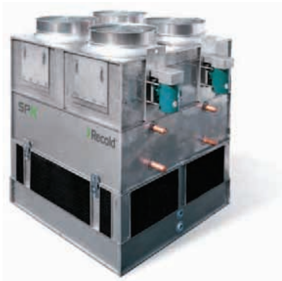
Recold MW Fluid Cooler —Induced draft, counterflow design. G-235 galvanized steel factory assembled structure. Also available in 300 series stainless steel. Proven copper coil technology.
