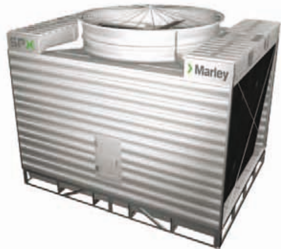
Marley NX Fiberglass Cooling Tower —Fiberglass and galvanized steel, field-erected, crossflow cooling tower designed to serve air conditioning and refrigeration systems. Cells available from 121 to 379 tons per cell. GB/T 7190.1-2000 Certified. Not available in the US, Canada or Europe.
