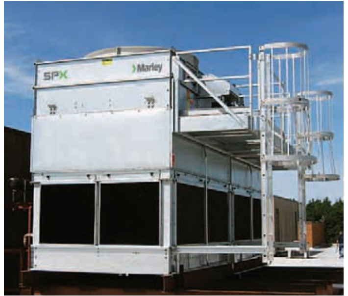
Marley MD Cooling Tower —Counterflow, induced-draft design requires less plan area than crossflow towers. Factory assembly and G-235 galvanized steel construction are standard. Tower available from 165 to 500 tons per cell. The all stainless steel option enhances the versatility of the MD. Five-year mechanical equipment warranty. CTI Certified.
