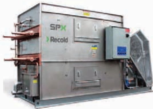
Recold JW Fluid Cooler —Forced-draft, low profile design. G-235 galvanized steel factory assembled structure. Also available in 300 series stainless steel. Proven copper coil technology.
