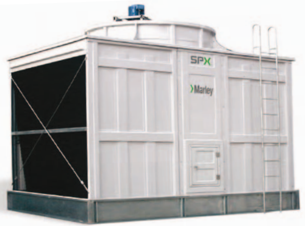
Marley NC® Fiberglass Cooling Tower —Fiberglass and galvanized steel, field-erected, crossflow cooling tower designed to serve air conditioning and refrigeration systems as well as light or medium industrial process loads on clean water. Stainless steel structure option available. Cells available from 105 to 942 tons per cell. CTI Certified. Not available in the US, Canada or Europe.
