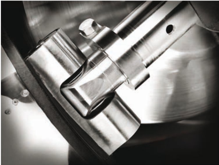
Fan blades are resiliently mounted to machined aluminum hub.
