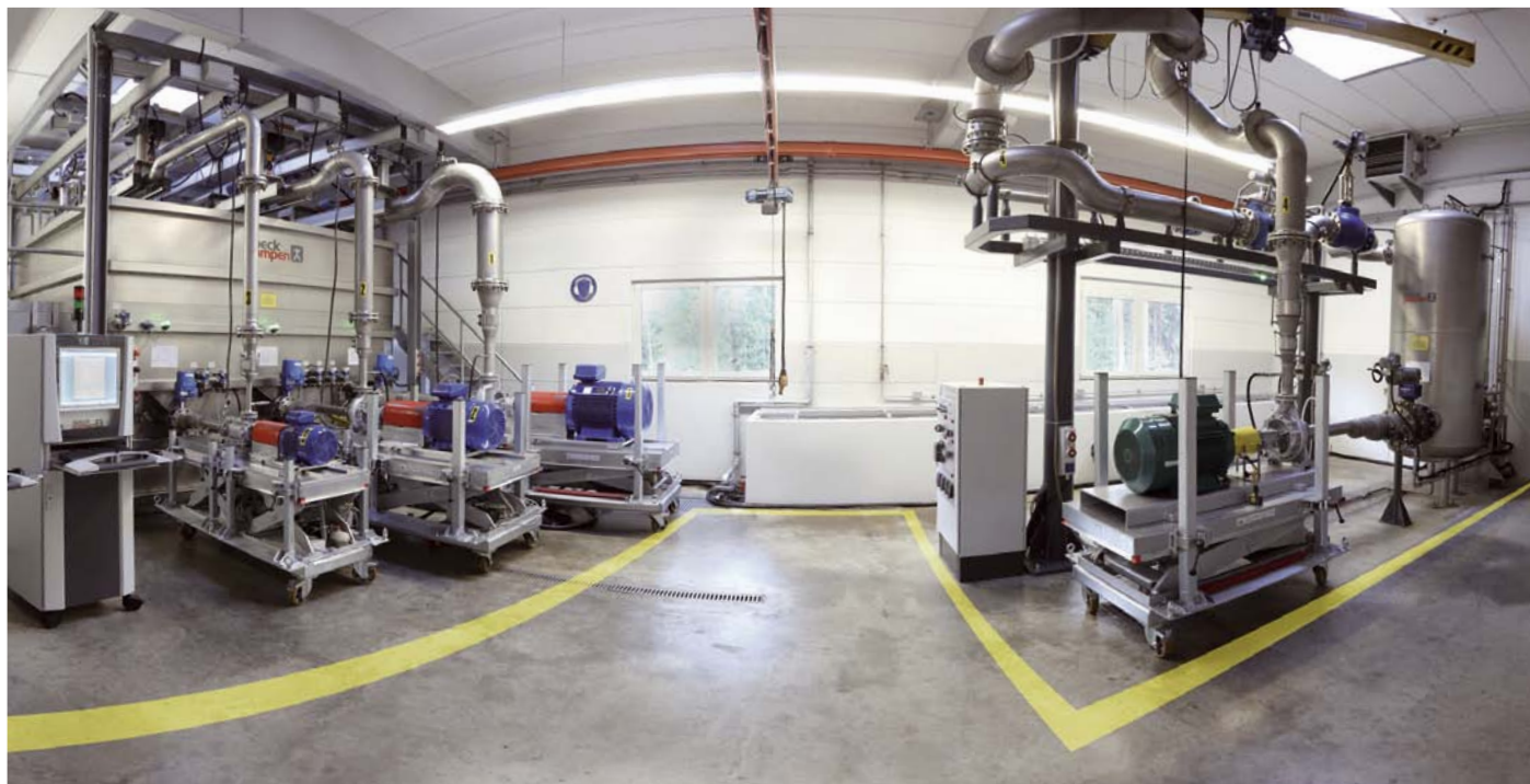
Test stand for liquid pumps on the premises of Speck in Roth Measuring of hydraulics, power requirements, axial thrust, vibrations and NPSH values. Heads of up to 400 m and flow rates of up to 750 m 3 /h.
