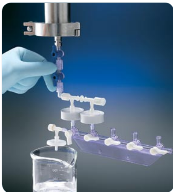
Performing bench scale Viresolve Prefilter area optimization trials.
